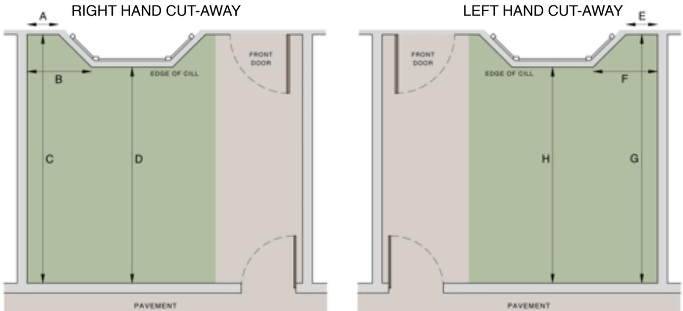
1. PLEASE RECORD DIMENSIONS **A,B,C** AND **D** IF YOUR BIKE SHED IS TO HAVE A **CUT-AWAY** ON ITS **RIGHT HAND SIDE** (LOOKING AT THE SHED FRONT ON)
